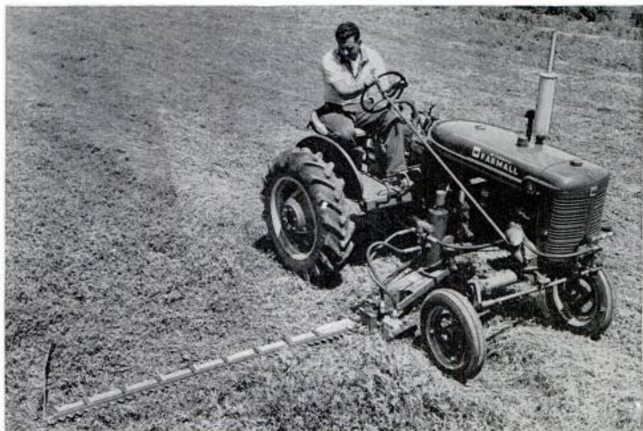
Commercial hydraulic mower operates at high speed and can be raised to any angle for ditch or hedge trimming
